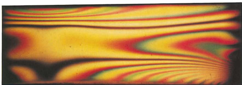
Fig. 3. Time dependent features. (a) Thermal instability in the lower boundary layer in the central portion of a wide roll. Pr = 440 , Ra_{\text{vertical}} = 10^5 and Ra_{\text{lateral}} = 3.3 \cdot 10^5 . The rising diapir is made apparent by weak horizontal isogradients. (b) Birth of a roll with large aspect ratio after the right hand side wall has suddenly been cooled ( Ra_{\text{lateral}} = 3.7 \cdot 10^4 ). The initial state is that shown in Figure 2 b. This shot is at time 100 sec. (c) Second shot 4 minutes after lateral cooling started. (d) Third shot at time 6 minutes. One approaches the steady state configuration with aspect ration 2.7.
