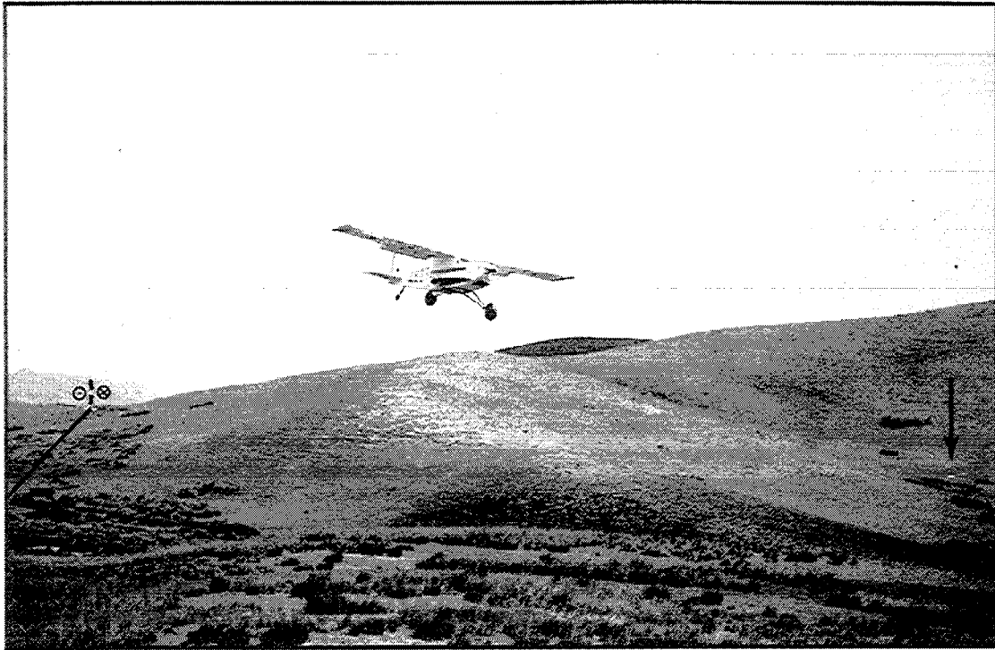
Figure 2. View of small remote-controlled airplane (3.3 m wingspan) flying above steppe along eastern swath (Figure 1a), before landing. Arrow points to one target used in stereopreparation of DEM (see discussion in text). Fault trace, on left side of photograph, is outlined.
