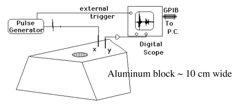
An impulse (with frequencies up to MHz) is applied at position x.
