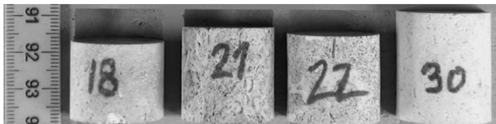
Fig. 2. Plugs 18, 21, 22 and 30 before compaction.
