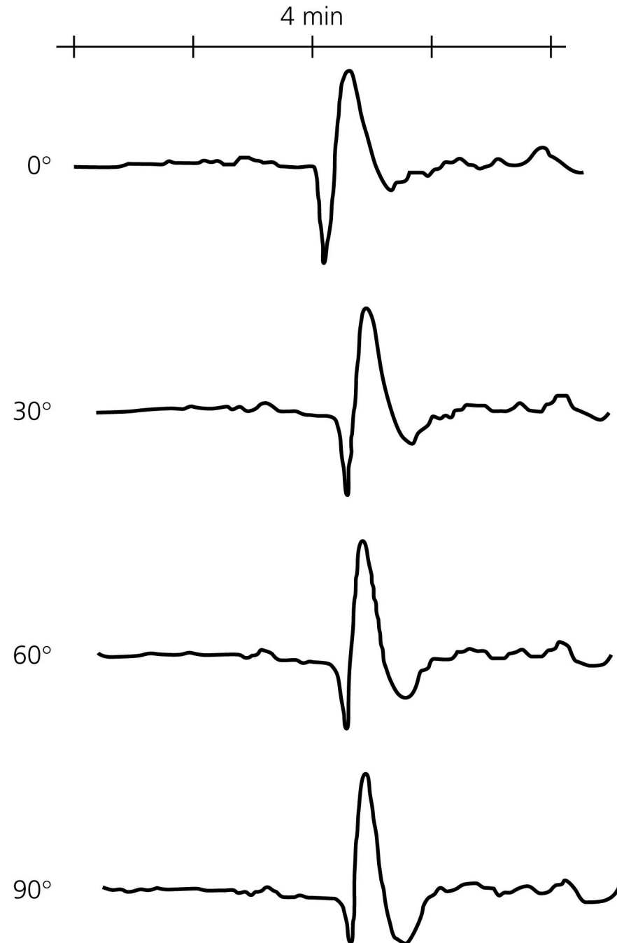
Figure 2.6-5: Effect of phase shifts on a seismic waveform.
