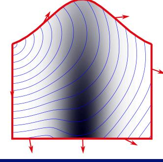
Domain boundaries and topography are handled by the weak formulation: an outgoing boundary condition is designed by the use of an additional flux term.
