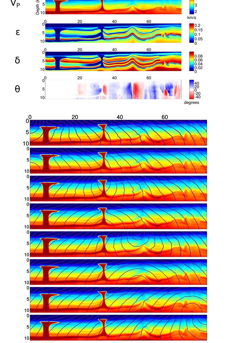
Traveltime isochrones for various source positions. Results from a FD code superimposed. 537600 degrees of freedom.
