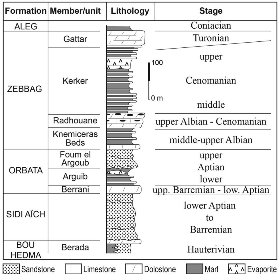
**Fig. 3.** Synthetic stratigraphic column of the Barremian–Turonian succession of the Chotts area, after Domergue et al. (1952) and Abbes and Tlig (1991).
