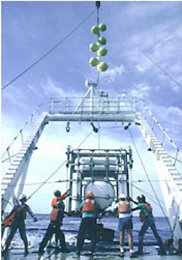
HLF-5 acoustic source (250 Hz) courtesy of Scripps Institution of Oceanography.
