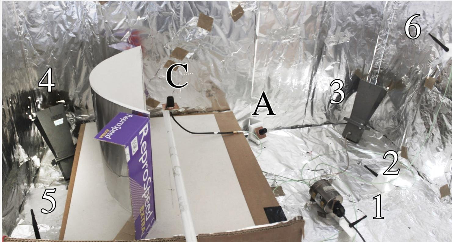
**Reverberation cavity** used in experimental set-up containing an **elliptic mirror** as a reflector, **emitting dipole** and horn **antennas (1-6)**, a **stationary receiver antenna (A)** and a **moving receiver (B)**; MIMO switch allows for successive emission from sources
