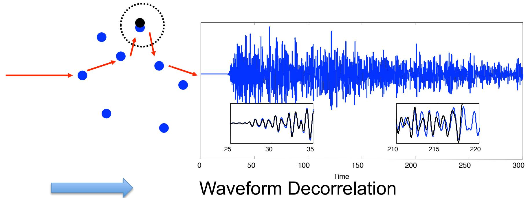
$$K^n(S, R, t) = 1 - \frac{\int \varphi_A(t) \varphi_B(t) dt}{\sqrt{\int \varphi_A^2(t) dt \int \varphi_B^2(t) dt}}$$
