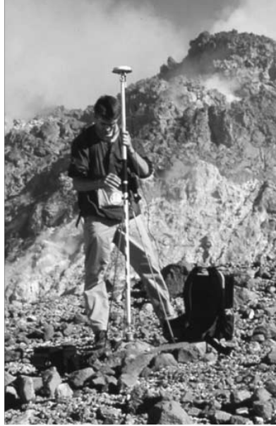
Figure 4.12: Kinematic GNSS acquisition at the AYI point (fig. 4.11). The receiver 2m-high antenna is positioned on the benchmark and stabilised by the operator. (From Beauducel et al. (2006))
