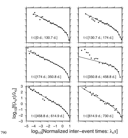
**Figure 6:** Adjustment of inter-event times distributions (dots) by a Gamma distribution (curve), according to a maximum likelihood method. Each subplot corresponds to the inter-event times distribution for a single time window with a constant background rate  $\lambda_0(t)$ . Time windows are defined by a change-point analysis, based on significant changes in successive inter-event time distributions (see section 4-1).
