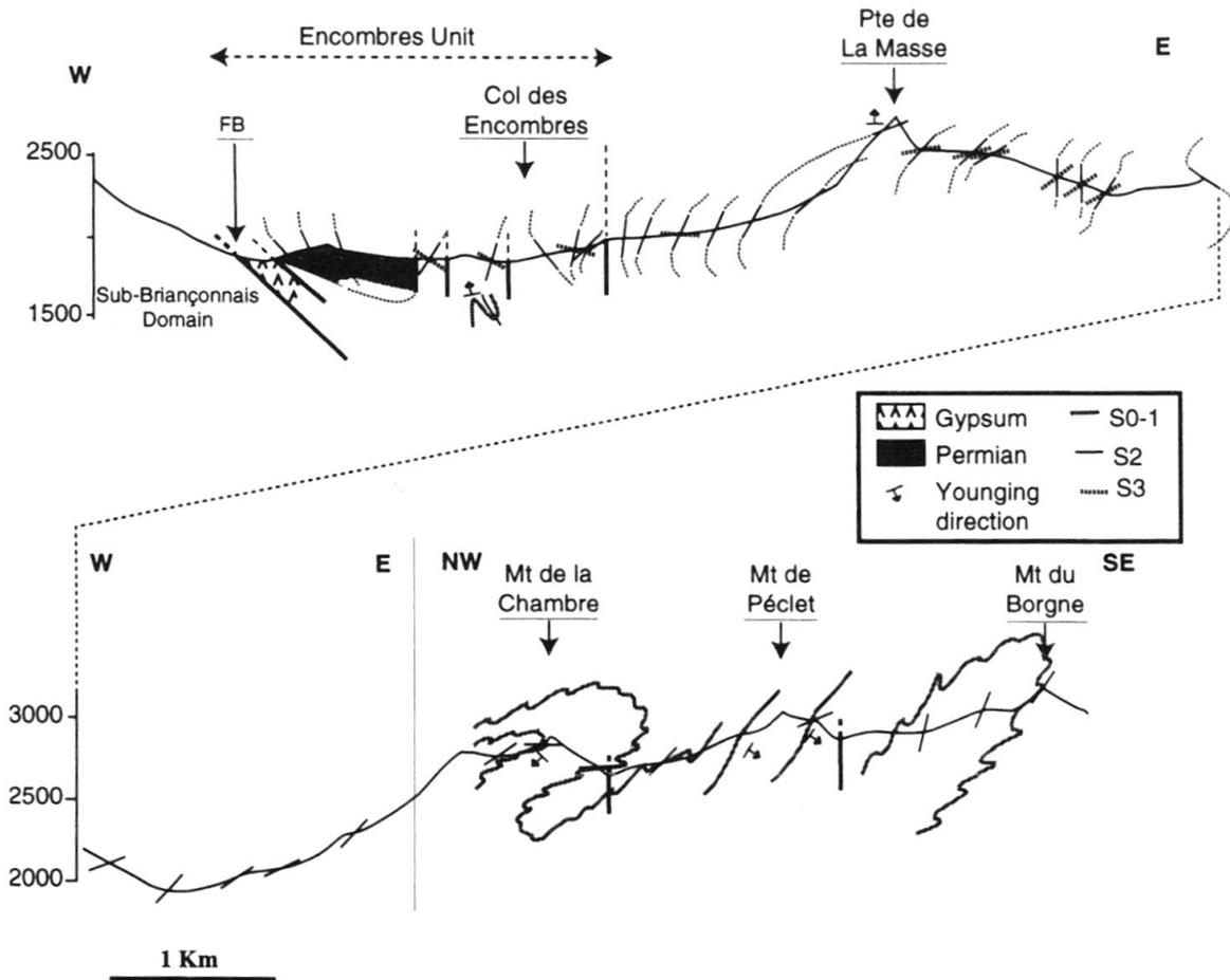
Fig. 4. Schematic cross-section of the ZHB stressing the attitude of the successive schistosités.
