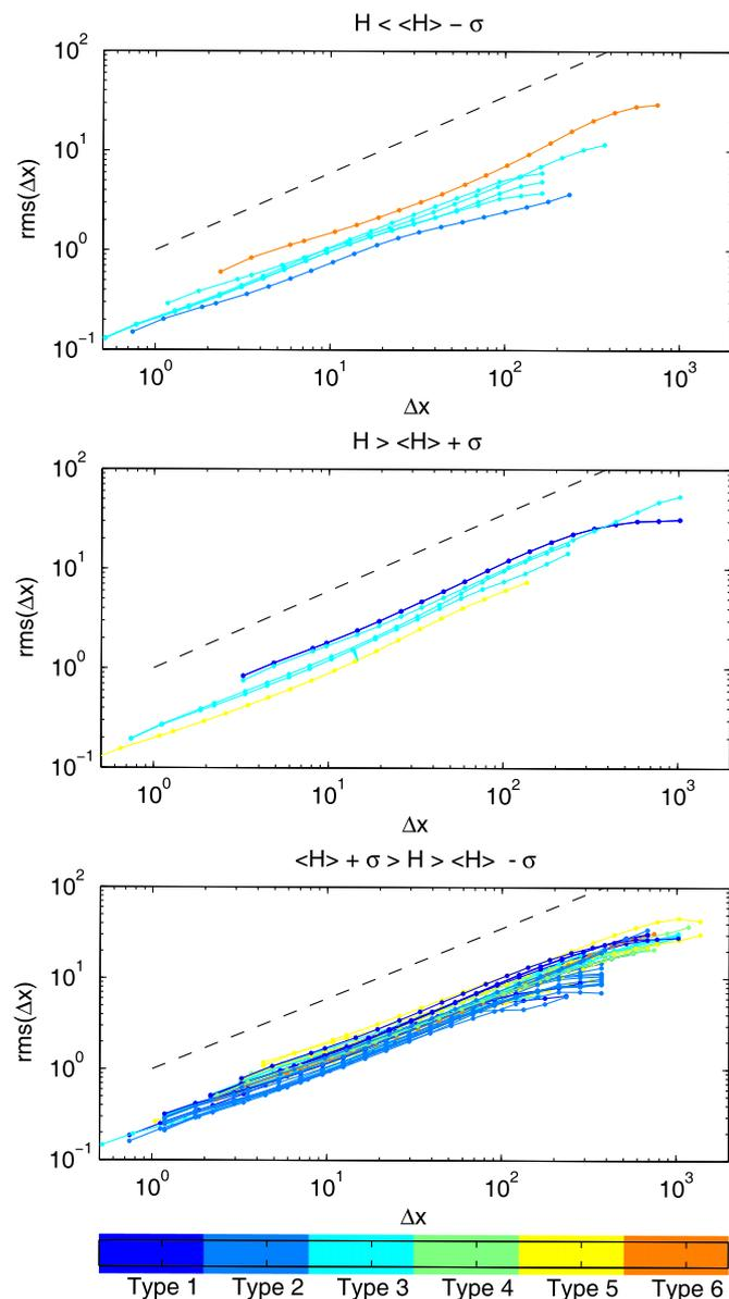
**Fig. 3.** Graphs representing the analysis of the Hurst exponent by the rms2 method. The fractures are divided into three groups; one (top) for those of Hurst exponent above one  $\sigma$  from the mean of the set, a second (middle) for those of Hurst exponent below one  $\sigma$  from the set mean, and a third (bottom) for those between one  $\sigma$  above and below the set mean. The dotted lines are given as guidelines and correspond to the mean value  $H = 0.78$ .
