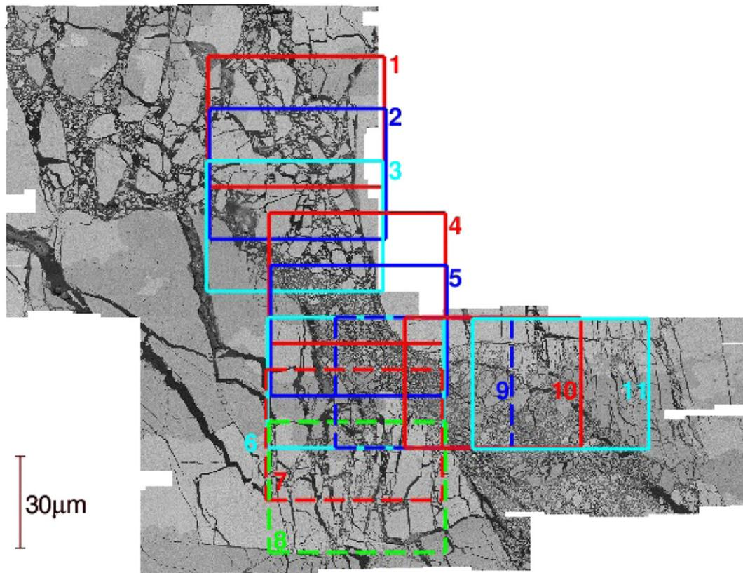
**Fig. 7.** Mosaic constructed from higher-resolution images of an extended area of image B from Fig. 6. Selected areas for particle size distribution analysis are outlined and labelled. The line types are selected only for clearer differentiation between rectangles and have no further significance. The direction of  $\sigma_1$  is parallel to the vertical edge of the image.
