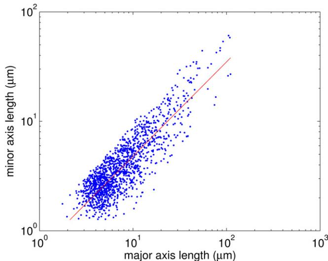
**Fig. 12.** Relation between the minimum axis and maximum axis lengths of the particles in the image A illustrated in Fig. 6. This figure serves as an example of the relation followed by the particles in all five images A–E.
