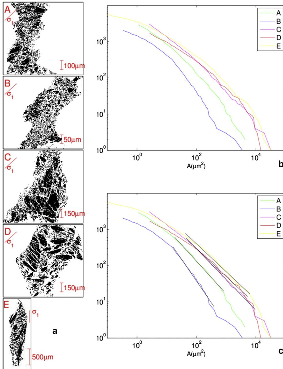
**Fig. 6.** Initial five shear zones A–E from the longitudinal thin section. a) segmented SEM images of the shear zones. b) corresponding particle size distributions. c) the same particle size distributions are shown with the power law fit superimposed, for exponents  $D_{2D>}$ .
