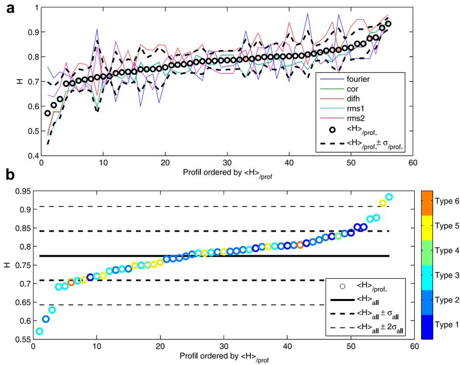
**Fig. 4.** All retained methods of calculation of the Hurst exponent represented individually, showing sufficient concordance of the Hurst exponent variation depending on method. a) The fractures are rank ordered by the mean Hurst exponent, which is then superimposed on the different methods, along with the standard deviations. b) The mean of the entire set of mean Hurst exponents, and one and two standard deviations either side of this are plotted with the individual mean Hurst exponents.
