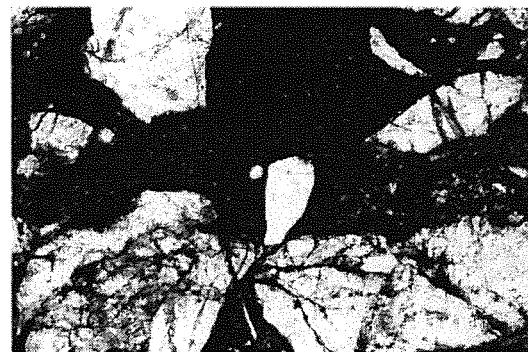
Figure 6. Microphotograph of the 622.6 m depth sample showing grey fragments of Si-cataclasite and quartz embedded in the black cement of the Ca-cataclasite. Thin section is horizontal in the core reference frame. Plane polarized light. Width of the view: 1.5 mm. - 622.6 m: This sample is almost completely cataclastic at the scale of the thin section. Both Si-cataclasites and Ca-cataclasites are observed. Fragments of Si-cataclasites are embedded in younger Si-cataclasites, and Si-cataclasites are themselves fragmented and embedded in Ca-cataclasite with highly variable percentage of carbonate cement. In the cement, euhedral crystals of carbonate may be observed within an unrecognized matrix, at high magnification on the petrographic microscope (see also description of fault gouge at 623.5m by Fujimoto et al., 1999).
