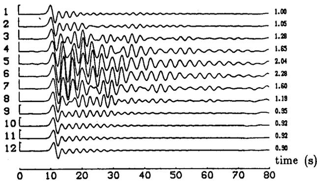
(b) Synthetic seismograms, at the same 12 sites, obtained when the clay pocket is taken into account.
