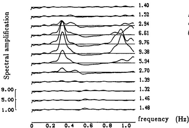
(c) Spectral ratios of signals shown in (b) with respect to the corresponding signals shown in (a).
