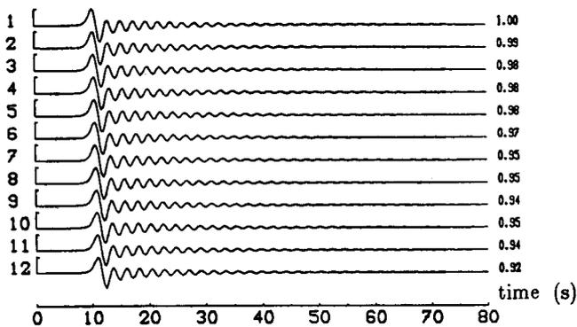
(a) Synthetic seismograms computed for a flat clay layer, at the same 12 surface sites as in Figure 12.
