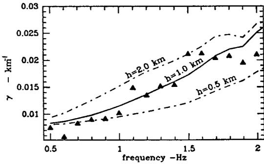
Fig. 6 Rg wave attenuation as a function of frequency for the data (triangles) and for three synthetic seismograms: model as described in table 1 (bold), models as described in table 1 but with a attenuative layer 0-2000 m (upper dashed - dotted) and 0-500 m (lower dashed - dotted).
