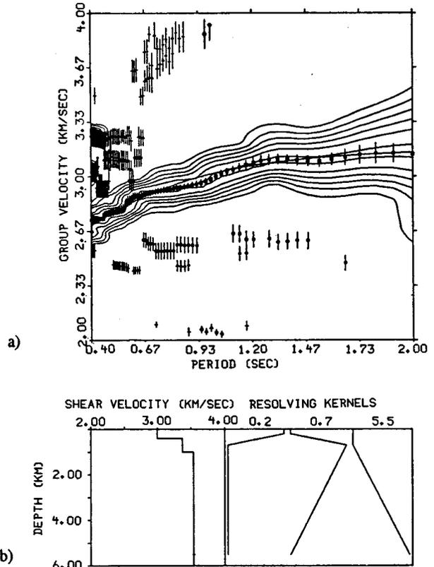
Fig. 3. a) Measured dispersion curve. Vertical bars indicate the standard deviation of the measure. The curve which corresponds to the earth model found by inversion of the dispersion curve is superimposed.
