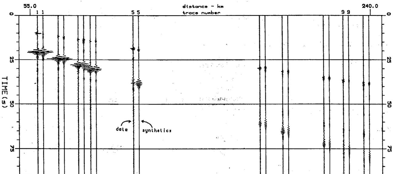
Fig. 5. Data (bold) and synthetic seismograms calculated for a crust with a 1 km thick attenuative surface layer. Both data and synthetic seismograms are bandpass filtered 0.5 - 2.0 Hz.
