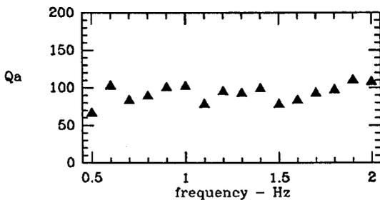
Fig. 4. The apparent quality factor  $Q_a$  as a function of frequency, found by linear regression as described in the text.
