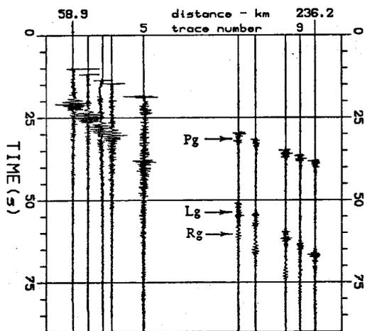
Fig. 2. The unfiltered records of the quarry blast.
