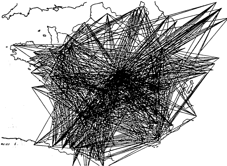
Fig. 3. Path coverage at a frequency of 3 Hz after sorting of the raw data.
