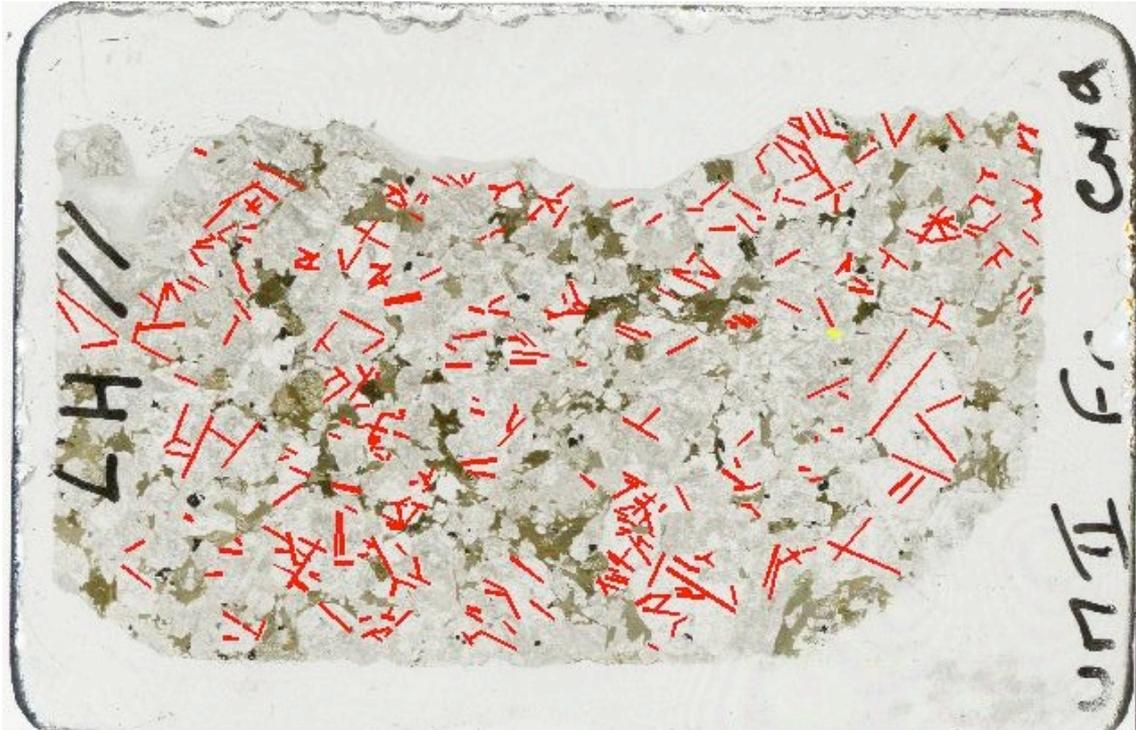
**Supplementary figure 7. Thin section of the granite used to make the samples.** Microfractures are highlighted in red. They are easily tracked in quartz but are much less obvious in altered feldspar and soft mica. The thin section is 4.5cm long and 3cm wide.
