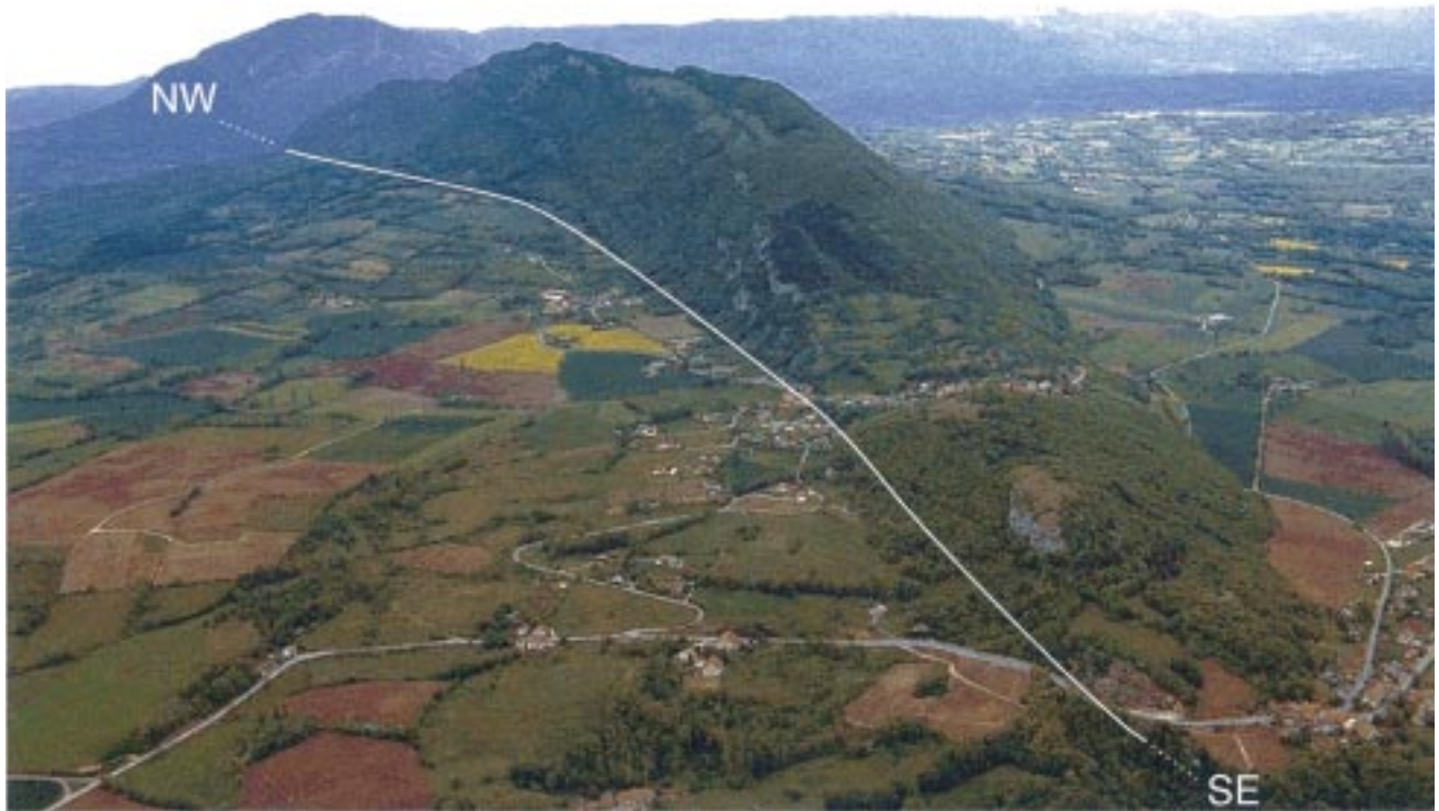
Figure 2. (a) Panchromatic Spot image (K-J/49-257, 1990-08-19) of the Vuache Fault (shown with arrows) between Lake Annecy (lower right corner) and Grand Cret d'Eau (upper left corner). E=Epagny (epicentre), MT=Metz-Tessy, M=Meythet, P=Poisy and Pr=Pringy denote NW suburbs of Annecy where most damage in the 1996 Epagny earthquake occurred; AV=Annecy-le-Vieux suffered less damage. (b) Structural framework and main recent faults of the area shown in (a) (dotted box). West-verging thrusts (dashed where hidden) underlie anticlines in the Mesozoic cover (dotted). The Vuache Fault joins Semnoz and Grand Cret d'Eau. (c) Airborne view of the Vuache mountain as seen from the SSW. The Vuache Fault trace is clearest at the southern foot of the mountain, roughly along the limit between forest and cultivated fields. Jura mountains in background.
