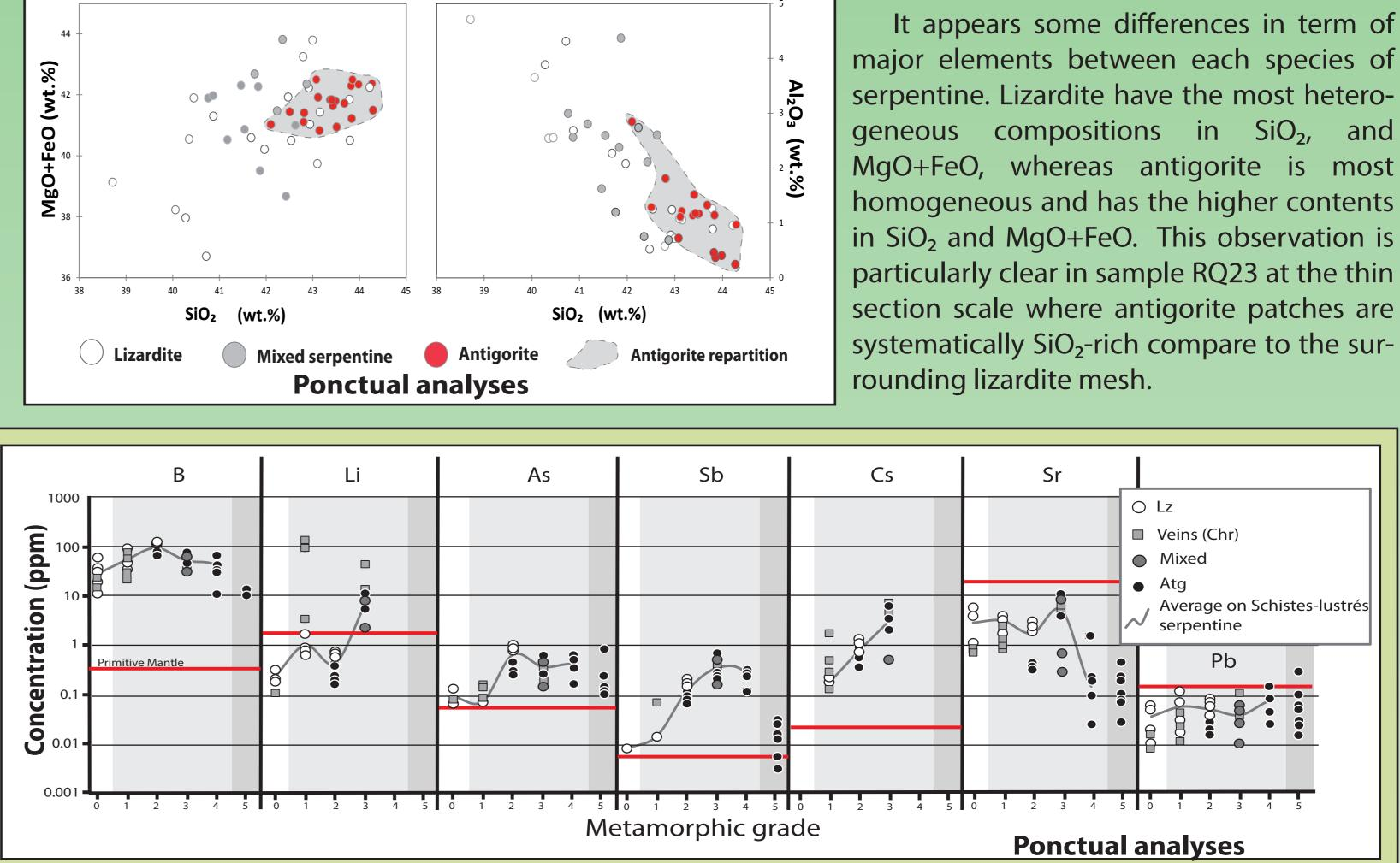
It appears some differences in term of major elements between each species of serpentine. Lizardite have the most heterogeneous compositions in SiO<sub>2</sub>, and MgO+FeO, whereas antigorite is most homogeneous and has the higher contents in SiO<sub>2</sub> and MgO+FeO. This observation is particularly clear in sample RQ23 at the thin section scale where antigorite patches are
