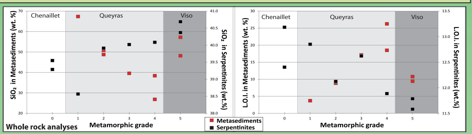
Serpentinites are relatively homogeneous in term of major elements. We assume that they derive from a protolith having depleted lherzolite composition. SiO<sub>2</sub> content is slightly increasing with metamorphic grade, whereas L.O.I. tends to decrease. This is the opposite for metasediments. Viso present the highest level in SiO<sub>2</sub> and the lowest L.O.I. in sediments and serpentinites. This underlines a strong dehydration of all the unit.
