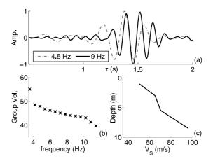
**Figure 2.** Dispersion analysis of the Rayleigh pulse. (a) The wave packet is filtered in two non-overlapping frequency bands (around 4.5 Hz and 9 Hz). (b) Observed dispersion curve of the Rayleigh wave group velocity. Dots: observations. Crosses: calculated data from the profile shown in (c). (c) Result of the inversion of the dispersion curve showing the upper 10 m of the shear wave velocity profile. See color version of this figure in the HTML.
