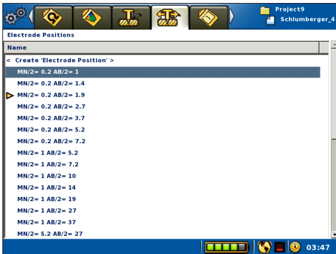
Figure 64. The Electrode Positions view in VES mode. Highlight on the second row and active electrode position marker on the fourth row
