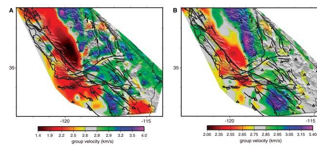
**Fig. 2.** Group-speed maps constructed by cross-correlating 30 days of ambient noise between USArray stations. (A) 7.5-s-period Rayleigh waves. (B) 15-s-period Rayleigh waves. Black solid lines show known
