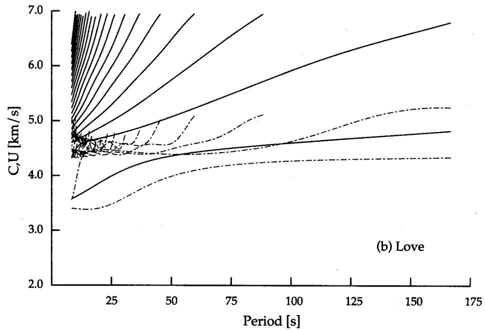
Figure 16.10. Dispersion curves for phase velocity  $C$  and group velocity  $U$  for the upper mantle of model AK135 as a function of period  $T$ : (a) Rayleigh waves, (b) Love waves. Phase velocity is shown as solid lines, group velocity as chain dotted lines in tone.
