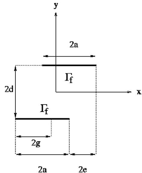
**Figure 3.** Fault geometry: two parallel segments of same half-length  $a$ . The input parameters are the half-separation  $d$  and the half-offset  $e$ . The half-length  $g$  of the effective slipping zone on the lower segment is an output of the calculations. In what follows, the top and bottom segments are called ‘upper’ and ‘lower’ faults, respectively.
