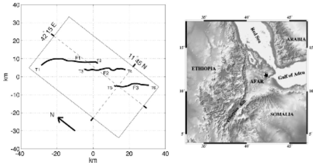
**Figure 11.** Fault system in Afar made of three *en echelon* normal fault segments. Inset shows general setting of Afar, and star locates the analysed fault system. Fault segments are denoted F1, F2 and F3 and fault tips T1, T2, ..., T6. This fault system geometry defines our geometrical support  $\Gamma_f = F1 \cup F2 \cup F3$  for the slip.
