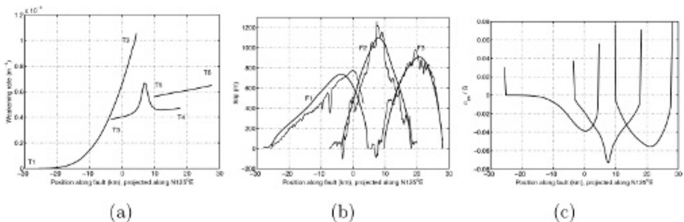
**Figure 12.** Results of the trial-and-error search for the three-faults system in Afar. From left to right, respectively: the deduced profiles of weakening along the faults, the computed slip profiles (thick lines) compared to the observed ones (thin lines), and the computed shear stress profiles on the faults.
