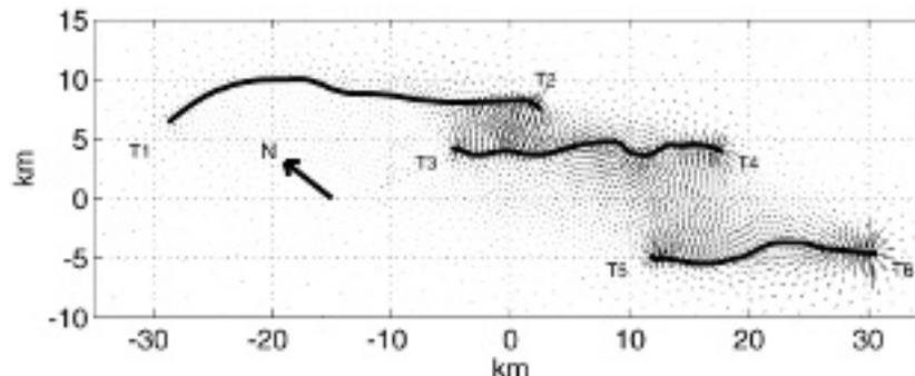
**Figure 14.** Orientation of the most solicited plane and unsigned magnitude of shear. At each point, the bar gives the orientation of the plane on which the shear stress is maximal, regardless of its sign. The length of the bar is proportional to the shear magnitude.
