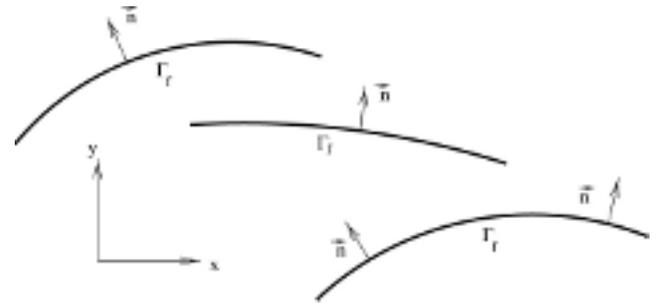
**Figure 1.** Antiplane normal fault definition. Fault segments lie in the  $xy$  plane. Their geometrical support is the segmented curve  $\Gamma_f$ . The local normal of  $\Gamma_f$  in the  $xy$  plane is denoted by  $n$ . Displacement  $u \equiv u_z$  and shear stresses  $\sigma_{zx}$  and  $\sigma_{zy}$  are perpendicular to the  $xy$  plane.
