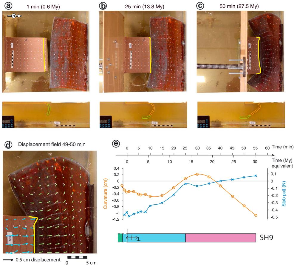
**Figure 5.** (a, b, and c) Top- and side-view photos of experiment SH9 at 1 min, 25 min, and 50 min, respectively. (d) Displacement field. (e) Timeline, curvature, and slab-pull evolution. Legend is the same as for Figure 3.
