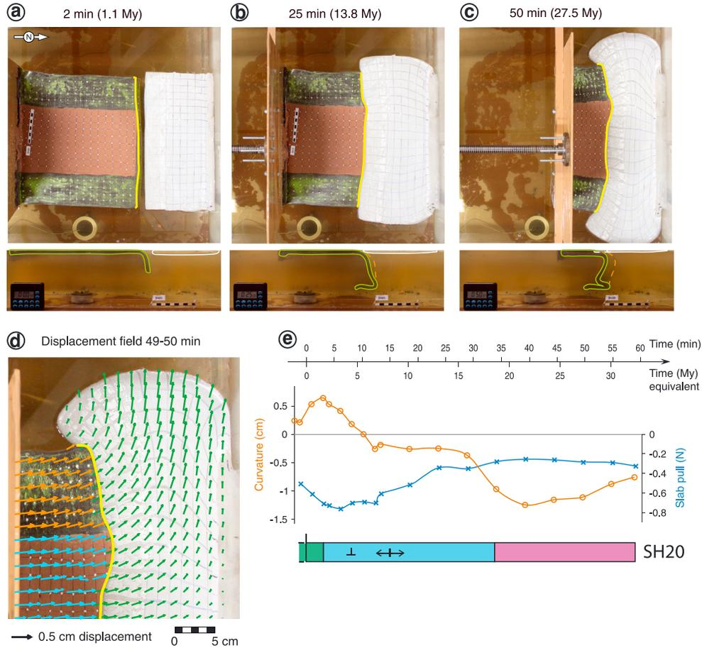
**Figure 9.** (a, b, and c) Top- and side-view photos of experiment SH20 at 2 min, 25 min, and 50 min, respectively. (d) Displacement field. (e) Timeline, curvature, and slab-pull evolution. Legend is the same as for Figure 3.
