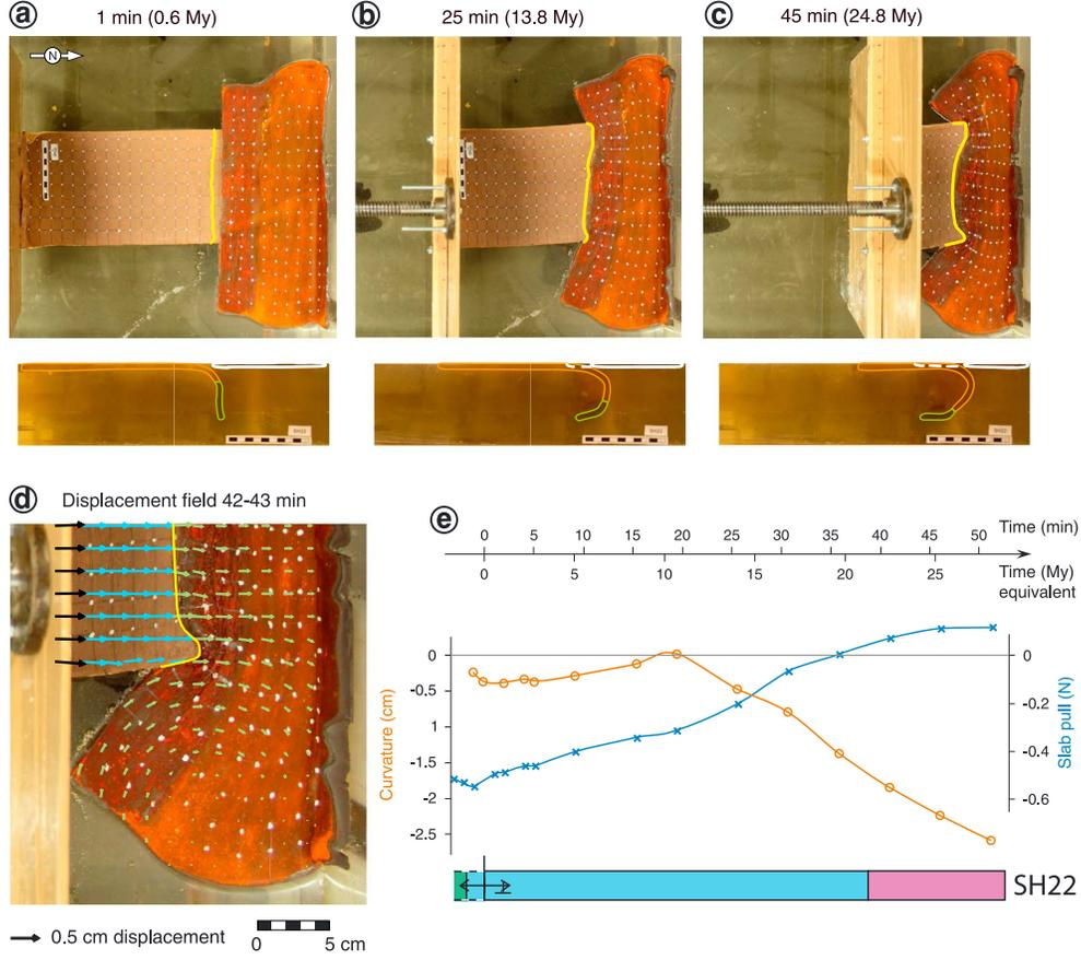
**Figure 4.** (a, b, and c) Top- and side-view photos of experiment SH22 at 1 min, 25 min, and 45 min, respectively. (d) Displacement field. (e) Timeline, curvature, and slab-pull evolution. Legend is the same as for Figure 3.
