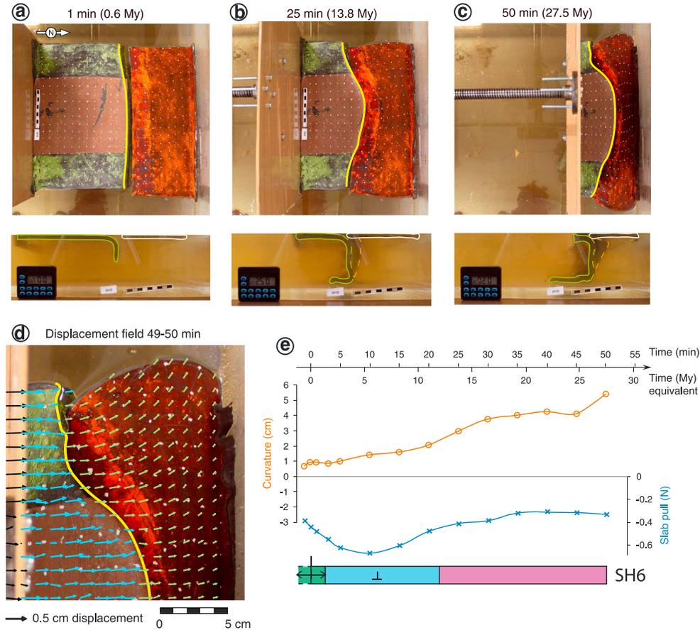
**Figure 8.** (a, b, and c) Top- and side-view photos of experiment SH6 at 1 min, 25 min, and 50 min, respectively. (d) Displacement field. (e) Timeline, curvature, and slab-pull evolution. Legend is the same as for Figure 3.
