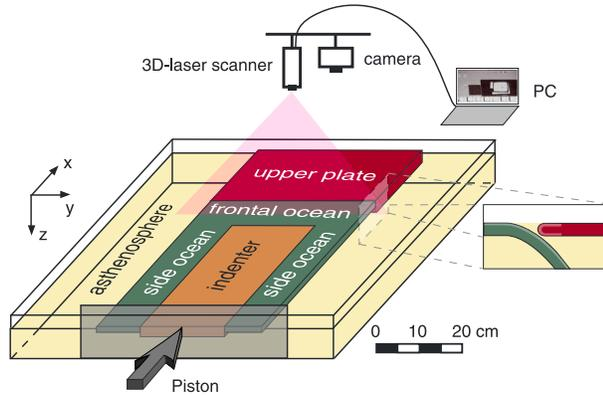
**Figure 2.** Experimental setup. Some experiments were performed only with the frontal ocean, others with both frontal and side oceans (Table 3). The subduction fault (plates interface) is lubricated with lubricant paste (petroleum jelly, in light colors), and glucose syrup is filling a small space between the plates, comparable to a weak zone.
