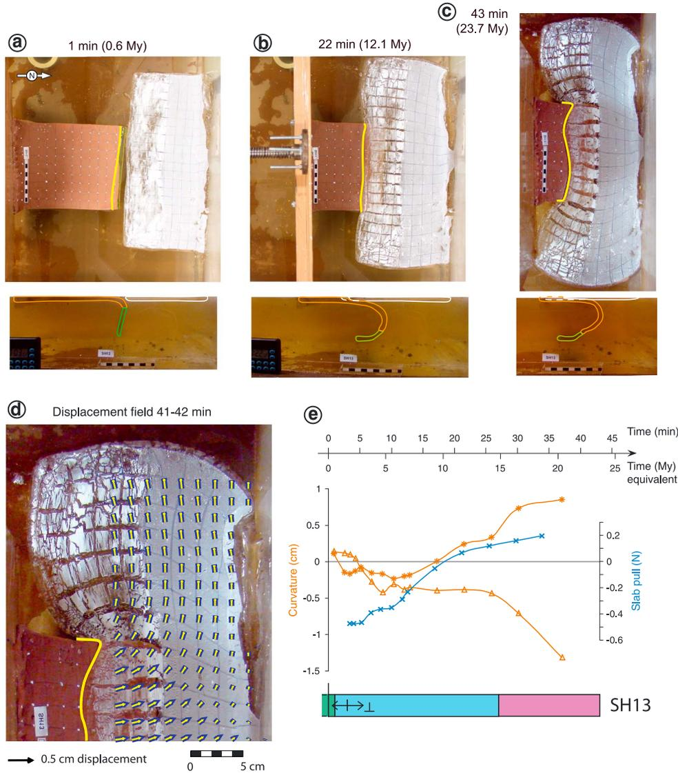
**Figure 7.** (a, b, and c) Top- and side-view photos of experiment SH13 at 1 min, 22 min, and 43 min, respectively. (d) Displacement field. (e) Timeline, curvature, and slab-pull evolution. Legend is the same as for Figure 3.
