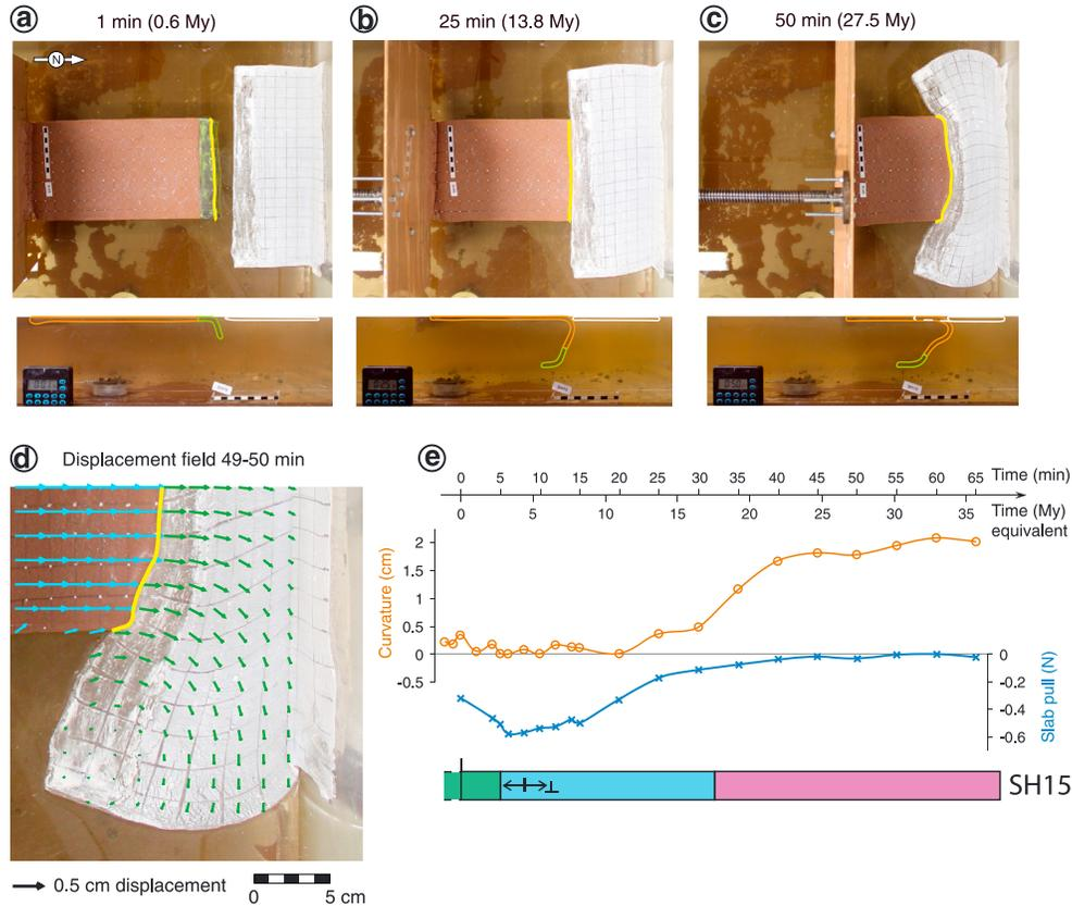
**Figure 6.** (a, b, and c) Top- and side-view photos of experiment SH15 at 1 min, 25 min, and 50 min, respectively. (d) Displacement field. (e) Timeline, curvature, and slab-pull evolution. Legend is the same as for Figure 3.
