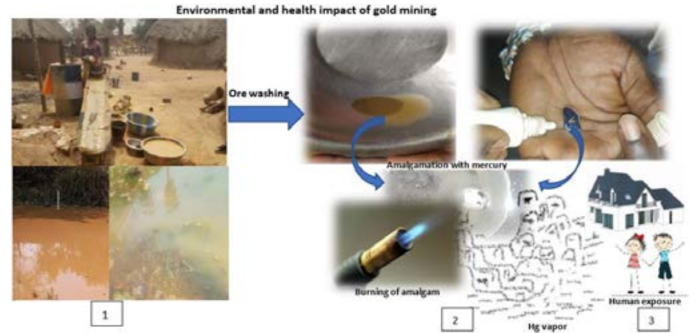
1- Ore washing and environmental impact of gold mining 2- Amalgamation of gold and burning of amalgam 3- Human exposure on Hg vapor
