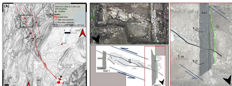
Fig 1: (A) Geomorphological imprint of the fault based on a 5-m-spatial resolution DEM, and on a 25-cm-spatial resolution DEM in the boxed area. Projected coordinate system: EPSG 2154, RGF93 / LAMBERT 93. (B): Area of archeoseismological investigations with a Zenithal view, and a structural diagram of the faulted zone. Focus (red box) on Wall 2 shows two phases of damage, 1: sinistral offset at the base and 2: tilting of the structure in the upper part.
