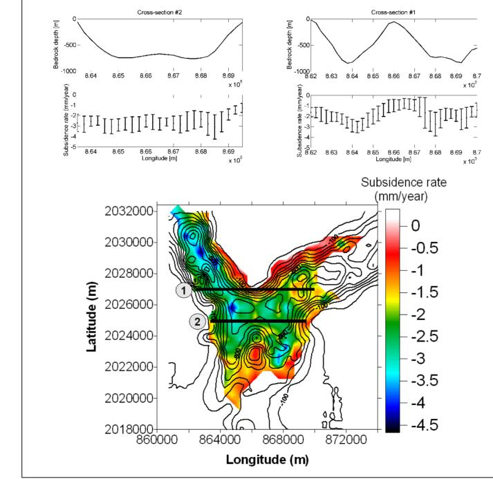
Bottom left figure displays a 500 m grid map of InSAR subsidence rates overlaid by the iso-contour lines of bedrock depth (in meters) while upper left figures show cross-sections of bedrock depth and subsidence rate:: higher is the bedrock depth, higher is the subsidence rate.
