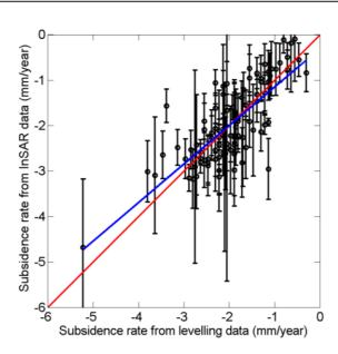
Comparison between subsidence rate derived from levelling and InSAR data is performed by averaging InSAR subsidence estimates in 200 m grid cells centred at levelling sites. Such size cells allow to account for most of the levelling data (100 over a total of 112 measurements) and a sufficient number of InSAR estimates (>5).
