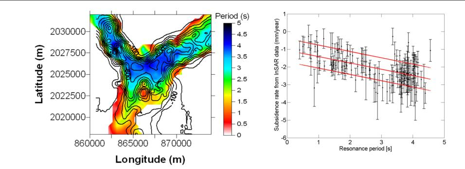
Left figure displays a 500 m grid map of H/V resonance periods overlaid by the iso-contour lines of bedrock depth (in meters) while right figure shows InSAR subsidence rates averaged over 200 m grid cells centred at the H/V site location. At first order, subsidence rate d is linearly correlated with the resonance period (T) through the following regression law:d (mm/an) = -0.36 T (s) -1
