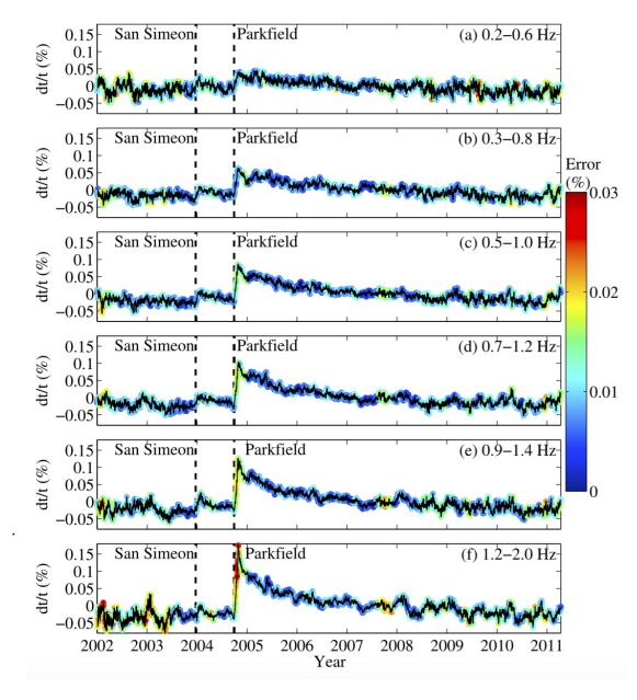
See velocity decrease after 2004 Parkfield earthquake, followed by slow recovery process. Change is largest at high frequencies, which are most sensitive to shallow changes in the upper few km (interpreted to be due to strong seismic shaking)
