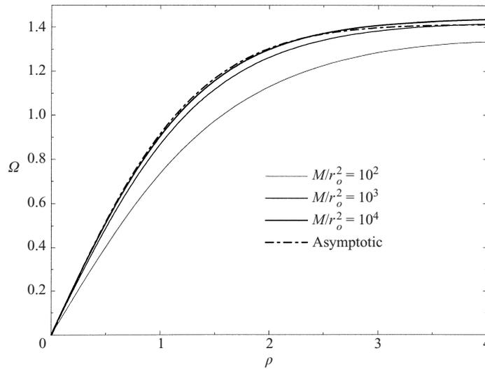
FIGURE 8. The angular velocity profiles  $\Omega$  plotted vs.  $\rho$  in the equatorial Hartmann layer on the equator  $\tau = 0$  for the radius ratio  $r_i/r_o = 0.35$ . The curves for  $M/r_o^2 = 10^2, 10^3, 10^4$  are identified by continuous lines of increasing solidity, which for small  $\rho$  approach the asymptotic solution (5.12) given by the short-long dashed curves.
