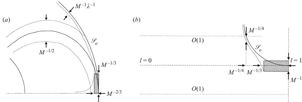
FIGURE 7. A schematic representation of the equatorial Hartmann layers and its neighbouring boundary layers on the outer-sphere boundary  $\mathcal{S}_o$ . Its relation to the  $M^{-1/2}$   $\mathcal{C}$ -shear layer and the outer sphere  $M^{-1}$  Hartmann layer are shown (a) in the meridional plane and (b) relative to the  $l, n$  boundary layer coordinates of the shear layer.
