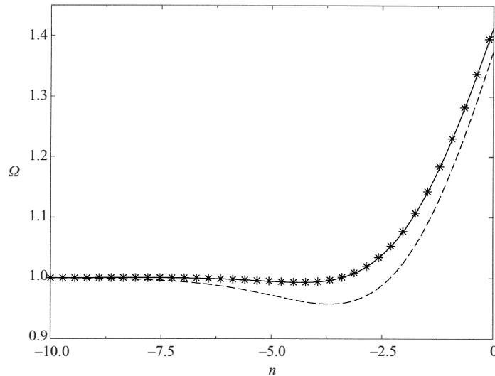
FIGURE 4. The angular velocity  $1 + \Omega_S(n)$  on the equatorial plane plotted *vs.*  $n$  in the narrow gap limit  $\varepsilon \ll 1$ . The dashed line denotes the two-term solution (3.18), the continuous line denotes its iteration to 100 terms and the stars denote the numerical solution of system (4.1).
