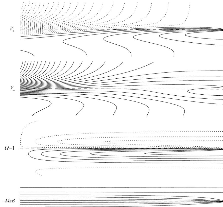
FIGURE 3. The numerical solution of the boundary layer equations (3.5a) in the  $l, n$ -plane for the radius ratio  $r_i/r_o = 0.35$  of figure 2. The  $l$ -axis  $0 \leq l \leq 1$  is identified by the horizontal dashed lines; the vertical extent is  $-15 \leq n \leq 15$ . As in figure 2, positive (negative) isovalues are indicated by the continuous (dotted) lines.
