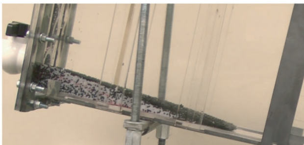
Fig. 3. Experiment with a slope less than 15°. No movement was observed after 1 h.
