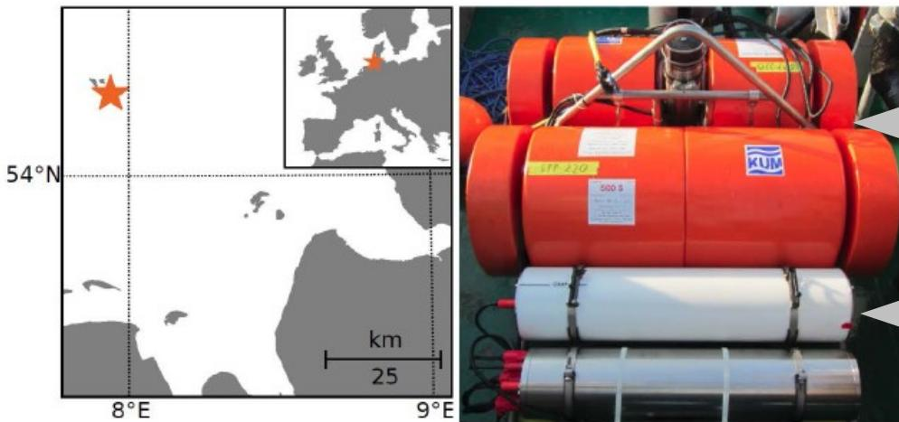
Seismometer (sensitive to tilt)
