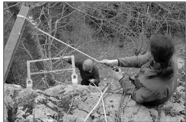
Figure 3. Photograph of GPR-data acquisition on a vertical cliff face (TE mode).
