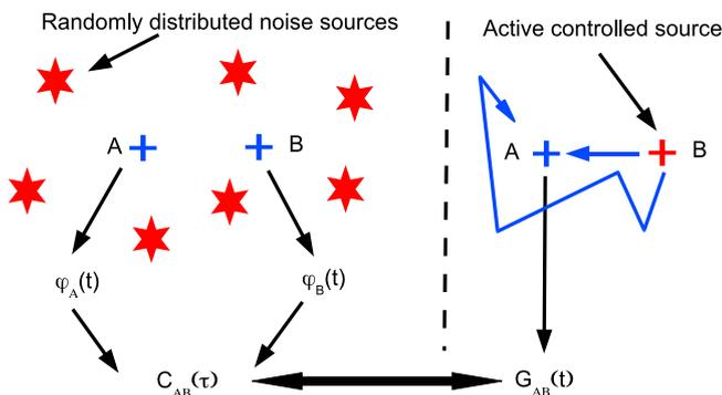
**Fig. 2.** Conceptual equivalence between passive experiment based on ambient noise correlation (left) and active experiment (right). Red stars: noise sources; blue crosses: receivers; red cross: controlled source. The correlation  $C_{AB}(\tau)$  between the two simultaneous records  $\varphi_A(t)$  and  $\varphi_B(t)$  yields the impulse response  $G_{AB}(\tau)$  provided that enough noise sources surround the receivers. Blue arrows: direct and multiply scattered (coda) waves.
