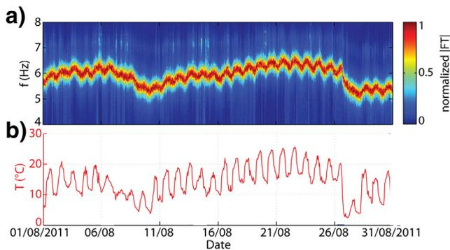
**Fig. 8.** a) Evolution of the natural resonant frequency of the rock column during summer (see Bottelin et al. (2013b) for more details on the data processing). (b) Temperature variations. Daily cycles are observable on both parameters, demonstrating the resonant frequency to depend on the external temperature.
