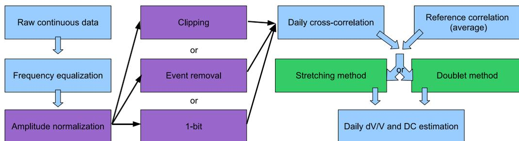
**Fig. 4.** General workflow to process ambient seismic noise correlation and extract daily relative velocity changes  $dV/V$  and decorrelation values  $DC$ .
