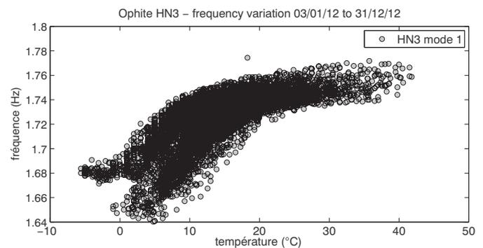
Fig. 6. Relation between the resonant frequency of the Ophite tower building and the outside air temperature in the transverse (HN3) direction. Only the first mode is displayed. Each dot corresponds to the frequency of the fundamental mode extracted using the Random Decrement Technique on window for 1 h applied to one year of data collected in 2012. Data were processed similarly to those collected in 2010 and published in ref. Mikael et al. (2013).
