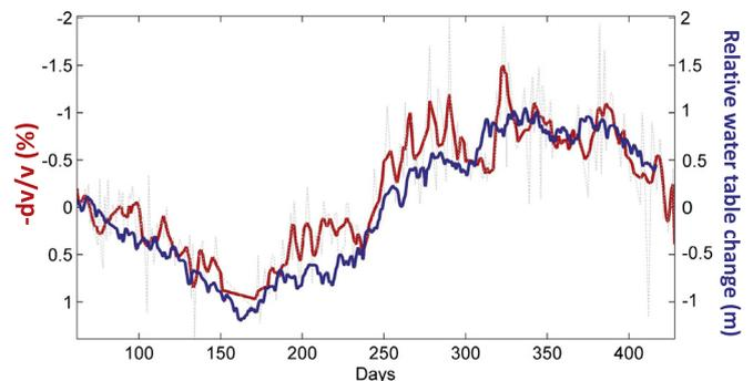
**Fig. 9.** Relative seismic velocity variations monitored at Utiku, New Zealand, in red, mostly in the 5–10 Hz range. Piezometric head levels are shown in blue. Data have been collected from late 2008 to early 2010. The relative positions of the seismic sensors were stable during the course of the experiment.
