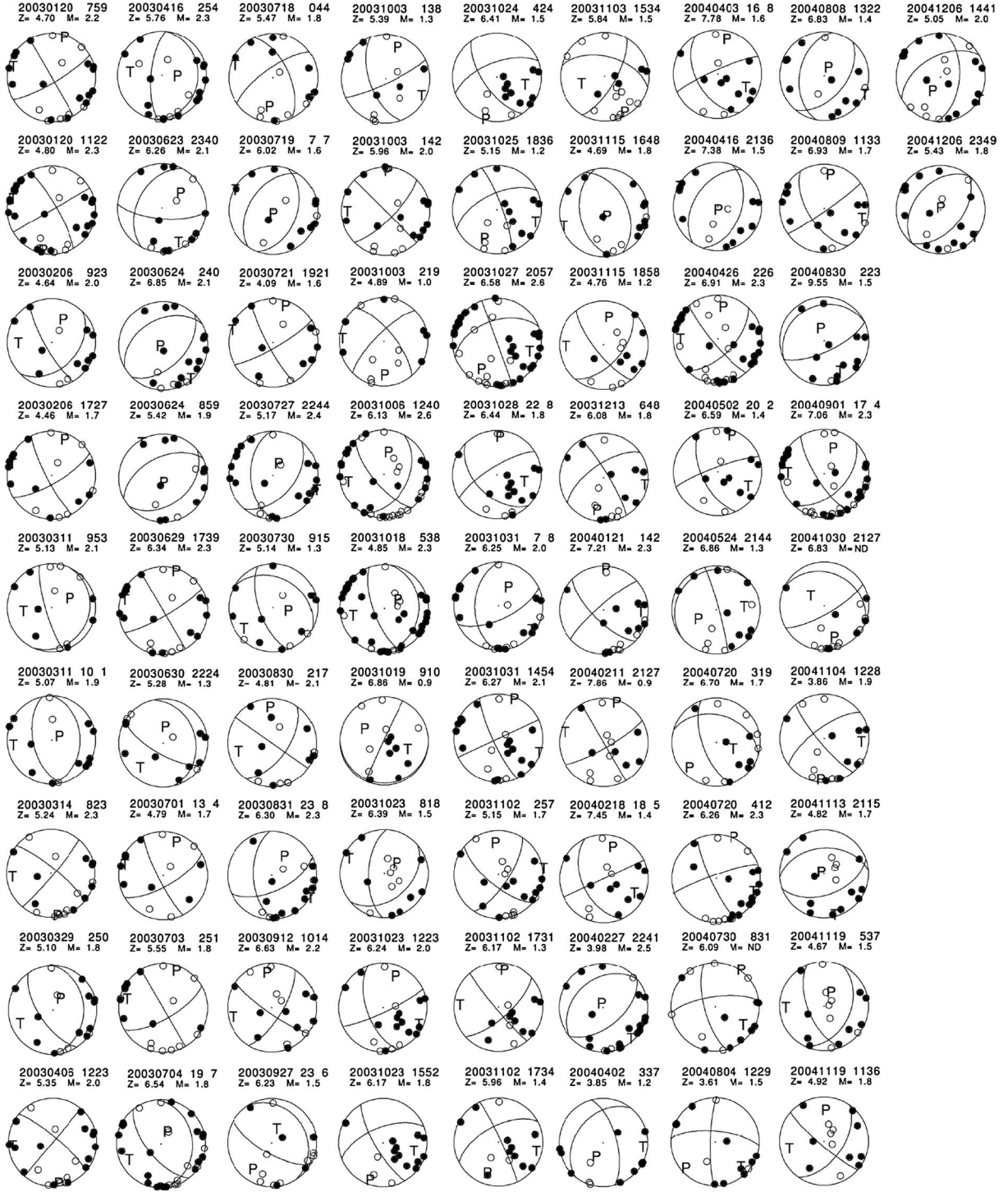
Figure 4. Focal mechanisms (lower hemisphere, equal area projection) for the 74 largest events of the Ubaye swarm. The heading over each diagram indicates the date, origin time, depth, and magnitude of the event.
