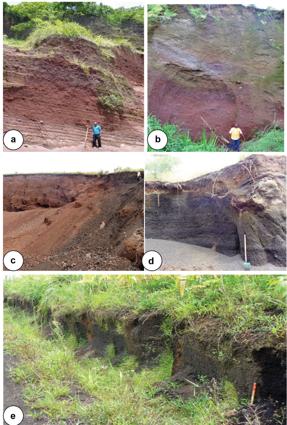
Fig. 2 Photographs showing some outcrops of the studied pozzolans. a Reddish to medium brown stratified deposits in the Tombel Plain; b Reddish to medium brown and Black pozzolan deposit surrounding Baleng Crater Lake in the Bamileke Plateau, c deposits showing an alternating beds of fine-grained “reddish” (dark brown) and coarse-grained black pozzolan at Foubot quarry (Noun Plain); d Uniform black pozzolan in front of Petpounoun lake (Noun Plain); e Dark yellow—colored pozzolans materials that constitute a soil of Monoun village (Noun Plain) and follows topography
