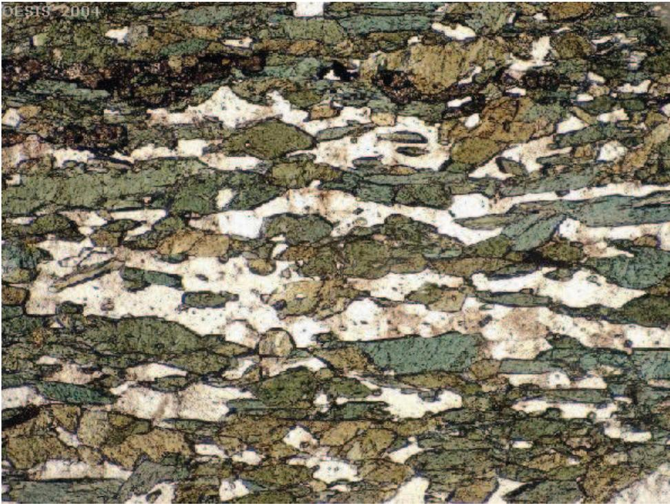
**Amphibolite.** This rock was originally a basic magmatic rock (basalt or dolerite). When metamorphosed, the heating and compression changed the original minerals to **hornblende** (green) and **feldspar** (colourless), and gave the rock a **banding** of minerals. Field of view 2 mm.
