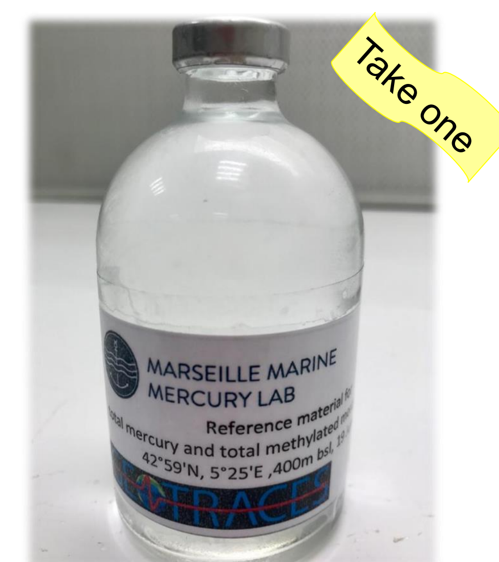
2017 GEOTRACES reference seawater for ambient tHg and MeHg concentrations
