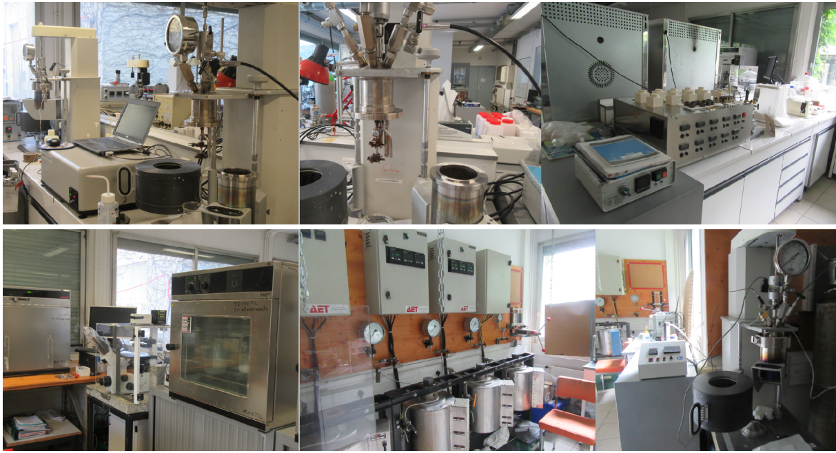
Figure 4. Experimental room for mineral-fluid interactions under mild and hydrothermal condition (up to 400°C and 500bar). All these experimental setups are also summarized in some slides available in my page web ( https://www.isterre.fr/IMG/pdf/experimental-setups-in-my-lab.pdf )
