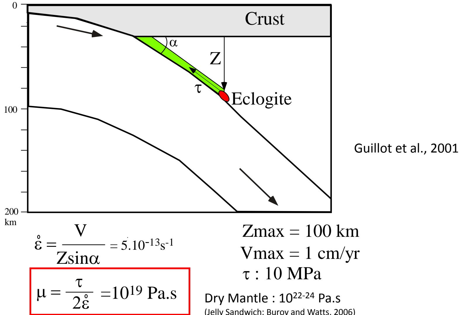
The viscosity and the density of the subduction channel should be low !!
