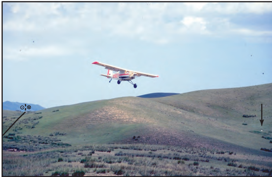
FIG. 2.3: View of small remote-controlled airplane (3.3 m wingspan) flying above steppe along eastern swath (Figure 2.2a), before landing. Arrow points to one target used in stereopreparation of DEM (see discussion in text). Fault trace, on left side of photograph, is outlined.
