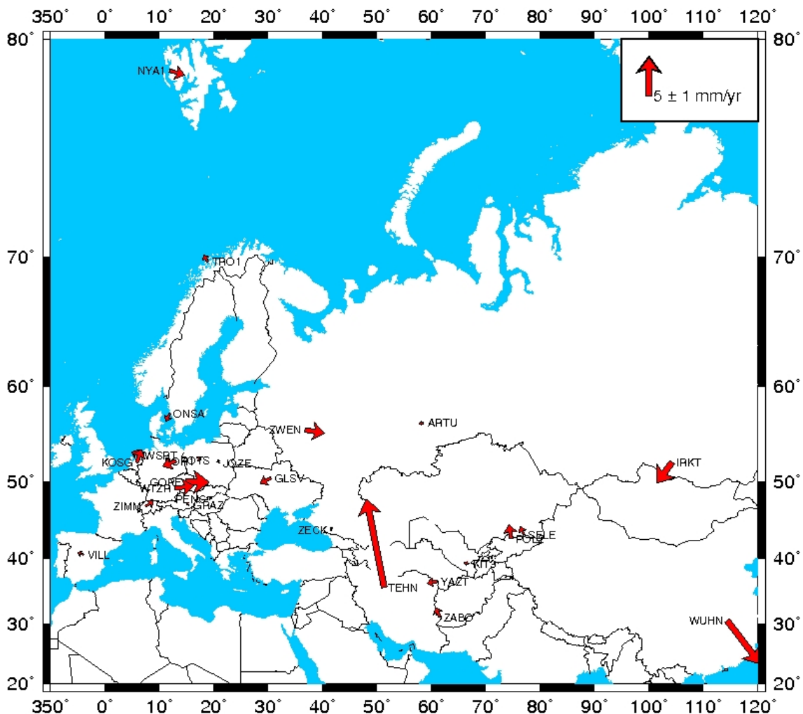
Figure 2-10. Velocity residuals of some European and Asian stations with respect to Eurasia. The velocities of the YAZT and the ZABO station in the east of Iran are less than 2 mm/yr which shows these stations are on the rigid Eurasian plate.
