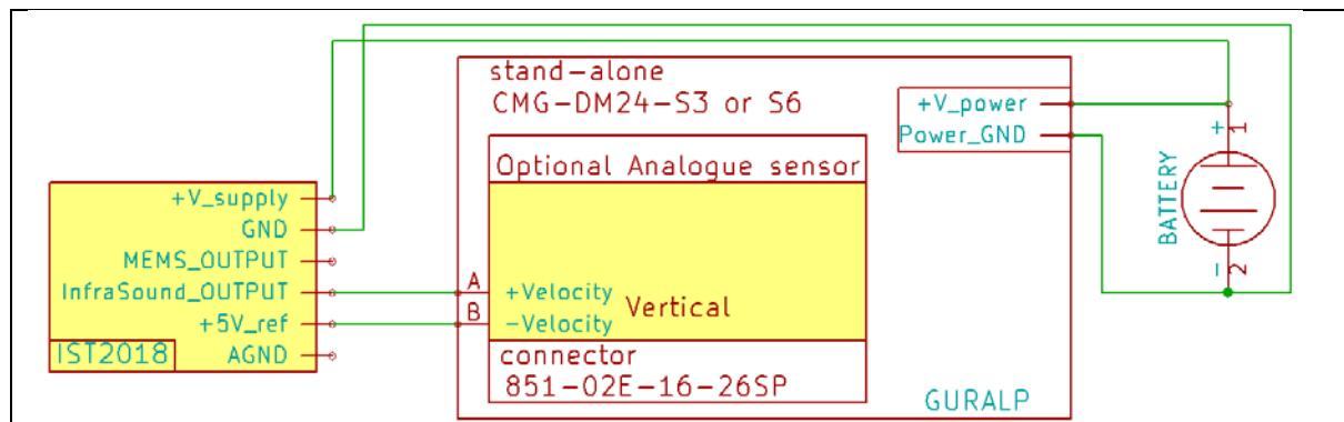
The only difference with §6.2.1 is that the ‘IST2018’ power supply is **directly connected to the battery**.
