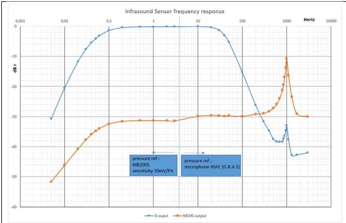
On the 'MEMS output' (red), the high pass filtering is produced by the pneumatic filter alone.
