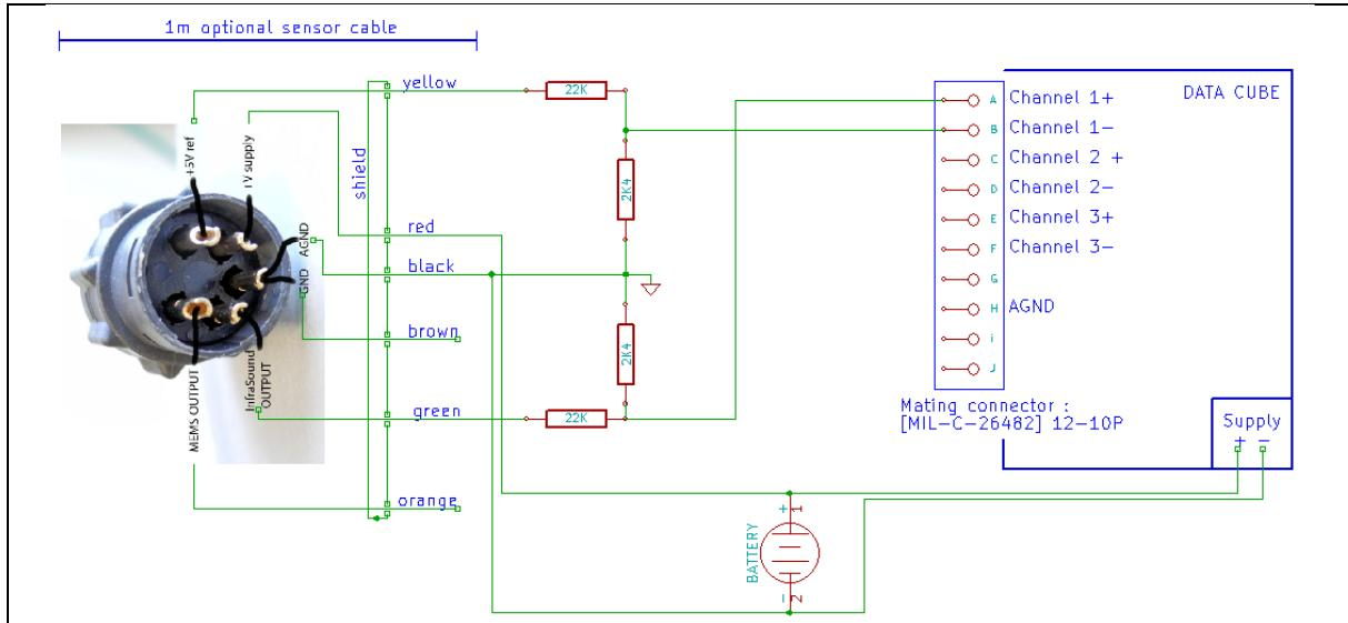
In this configuration (resistors divide the signal by 10), we obtain:
