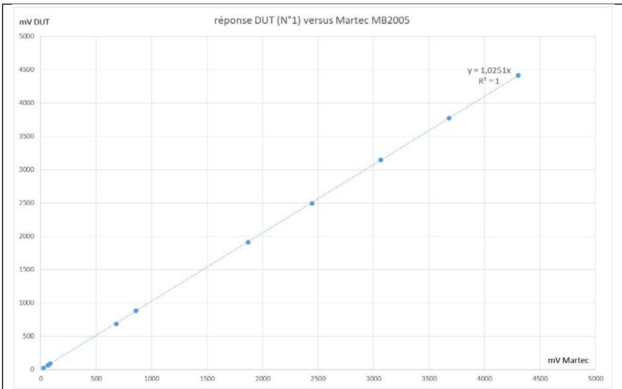
The linearity is good with respect to the MB2005 sensor, with a mean relative deviation of 0.66 %. (Measured on 'IS output' between 1.2Pa and 220Pa).
