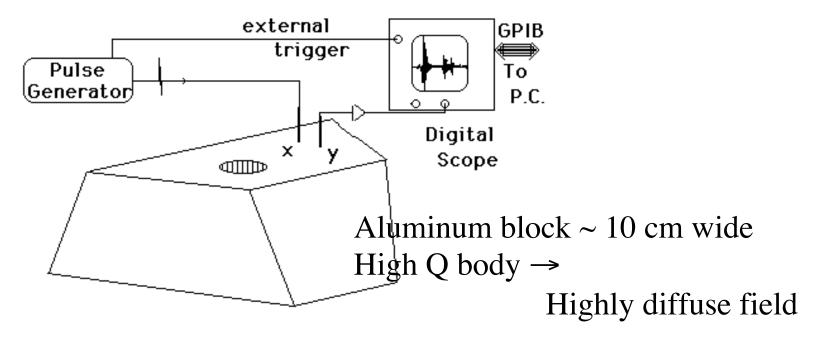
An impulse (with frequencies up to MHz) is applied at position x.
