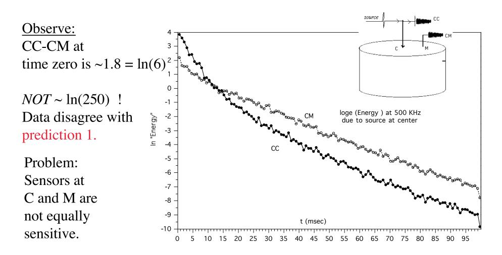
Fix(?) Calibrate by assuming (prediction 2) that at *late time* the ultrasonic energy densities at C and M are equal (i.e equipartition is achieved as  $t \rightarrow \infty$ )
