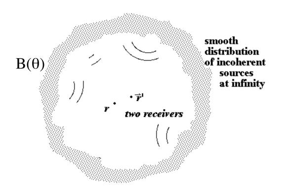
It produces a diffuse Intensity distribution  $B(\theta)$  incident upon a region containing our two receivers The field in the vicinity of the origin is a superposition of plane waves
