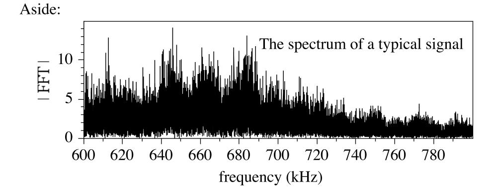
Note the undulations in the spectrum ~ frequency scales of O(20 kHz) correspond to times scales of O(50 µsec) = Transit times!
