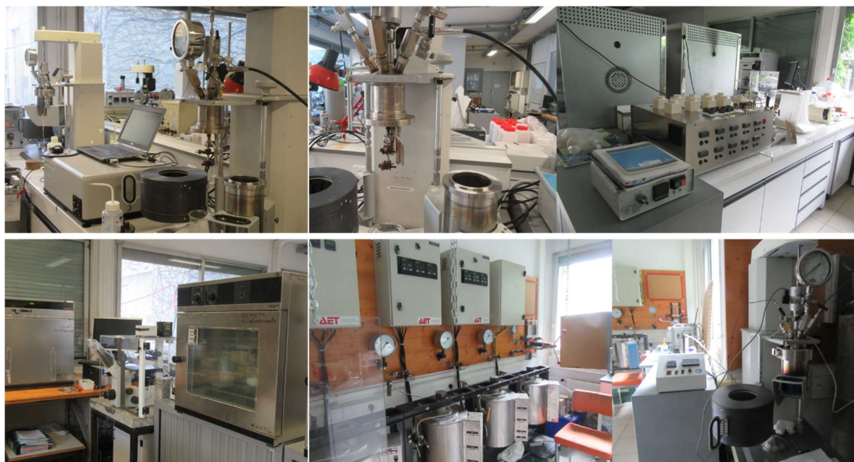
Figure 6. Experimental room for mineral-fluid interactions under mild and hydrothermal condition (up to 400°C and 500bar). All these experimental setups are also summarized in some slides available in my page web ( https://www.isterre.fr/IMG/pdf/experimental-setups-in-my-lab.pdf )
